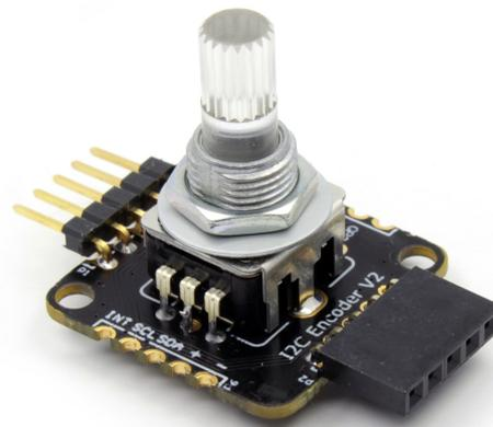
Figure 1.11: Example of assembled board with Illuminated RGB Encoder and connectors
