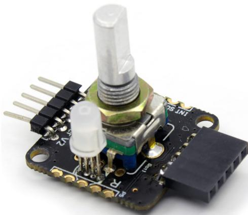
Figure 1.10: Example of assembled board with EC11 encoder, RGB LED and connectors
