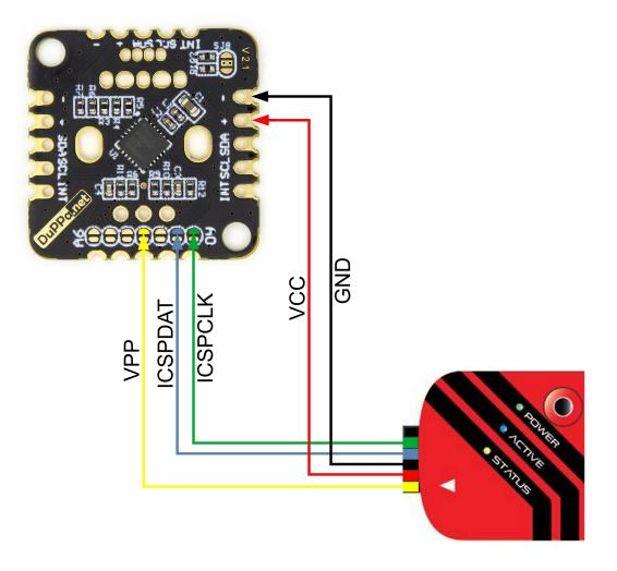
Figure 4.1: Schematic for programming with the PICkit 3
