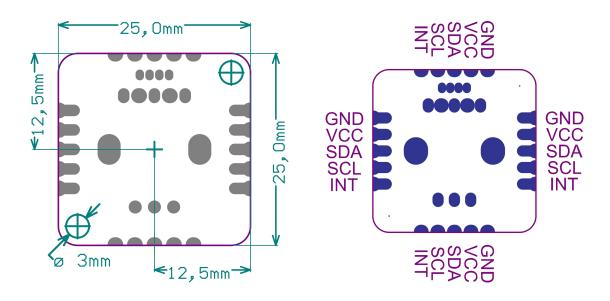
Figure 1.4: Dimensions of the board
