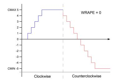
Figure 1.14: Blue and red line are the CVAL values when the encoder is rotate and the WRAPE is disabled
