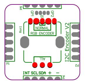
Figure 1.13: Used pins for mounting the RGB encoder  $% \left( {{\left[ {{{\rm{GB}}} \right]}_{\rm{COM}}} \right)$
