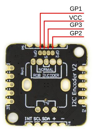
Figure 1.16: GP pins pinout
